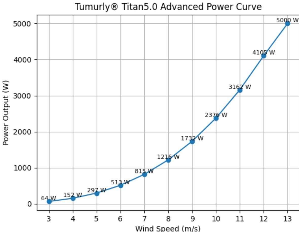
The Tumurly® Titan5.0 is an advanced 5.0 kW wind turbine developed through extensive R&D to deliver high efficiency and reliable performance. Rated at a wind speed of 13 m/s, the turbine features a 3.8 m rotor diameter and a swept area of 11.34 m<sup>2</sup>, achieving efficient energy capture with a power coefficient (Cp) of 0.38 under standard air density conditions (1.225 kg/m<sup>3</sup>).
